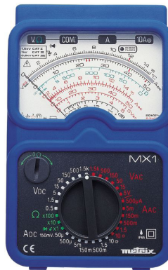
MX1 Analogue Multimeter 200A ac 1.5kV
